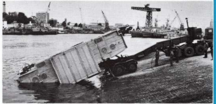
Launching trials on a ramp with a slope higher than 20 % Hundimiento sobre rampa superior a 20 %
